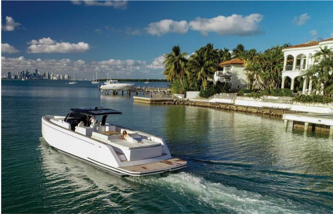
The transom sun pad measures 7 feet, 6 inches wide. High gunwales and 30-inch-wide side decks are designed for safe transit around the yacht. Courtesy Pardo Yachts
