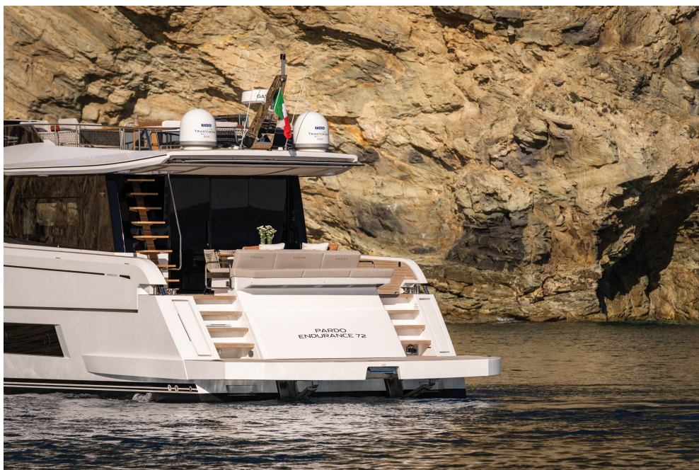
The Endurance 72 has a hydraulic swim platform and aft garage to accommodate up to a 12-foot tender. Courtesy Pardo Yachts
